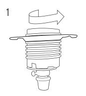
Adjust the metal ring so that it sits two threads into the socket. Align the knobs in the ring with the widest part of the shade.
