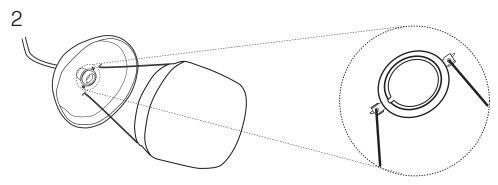
Install a compact LED lamp. Insert the metal barbs into the holes in the metal ring. Position the lamp shade so that it fits snuggly. Adjustments for a better fit can be made by threading our unthreading the metal ring in the socket.
