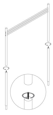
Screw the bottom wooden dowel sections into the top wooden dowel sections. Do not over tighten.
