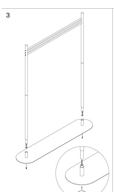
Carefully insert the assembly into the base. Tip the structure and carefully insert the base screws. Secure with the base screws using the allen wrench. Do not over-tighten.
