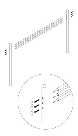
Carefully insert the cross bars into the holes on the top dowel sections. Lay them on the floor for easier assembly. Secure them with the six hex screws provided. Do not over-tighten them.
