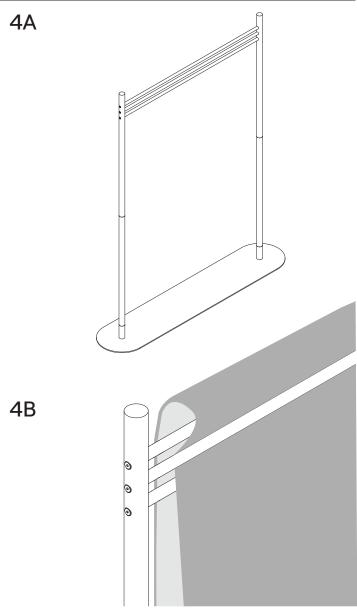
Once the assembly is complete position the frame where you want the divider. Insert the acoustic Quiltforms by threading them between the middle bar and draping it over the top bar. Steam out wrinkles and unevenness out of the Quiltforms.
