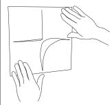
Apply tiles to surface, pressing each firmly, making sure that all corners are in contact with the surface.
