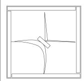
Apply tiles to surface pressing each tile firmly. Make sure that all edges are in contact with the surface and that tiles are securely adhered.
