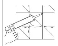
Use Fuze\*It to seal the seams. Clean up and smooth as you go along before it sets. Tiles should not be sanded. 8 (Required for painting tiles.)
