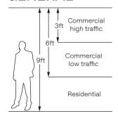
Make your installation last by applying tiles at a height that makes sense for the environment. Prevent tile damage and keep your Plasticforms looking beautiful.
