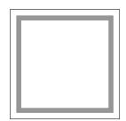
Apply a 1/4 inch adhesive bead to tile perimeter. Apply 1/4 in away from edge to prevent adhesive squeeze-out. Carefully remove and clean excess adhesive.
