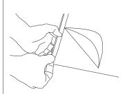
Apply the selected adhesion method to the perimeter and the center of tile when possible. We recommend 3M mounting tape.
