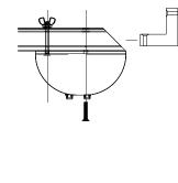
Use the shorter screw to secure the caster base into the threads in the frame.
