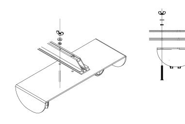
Align and secure the short extrusion with four holes at the bottom to the caster base using the long screw, wingnut and washers.
