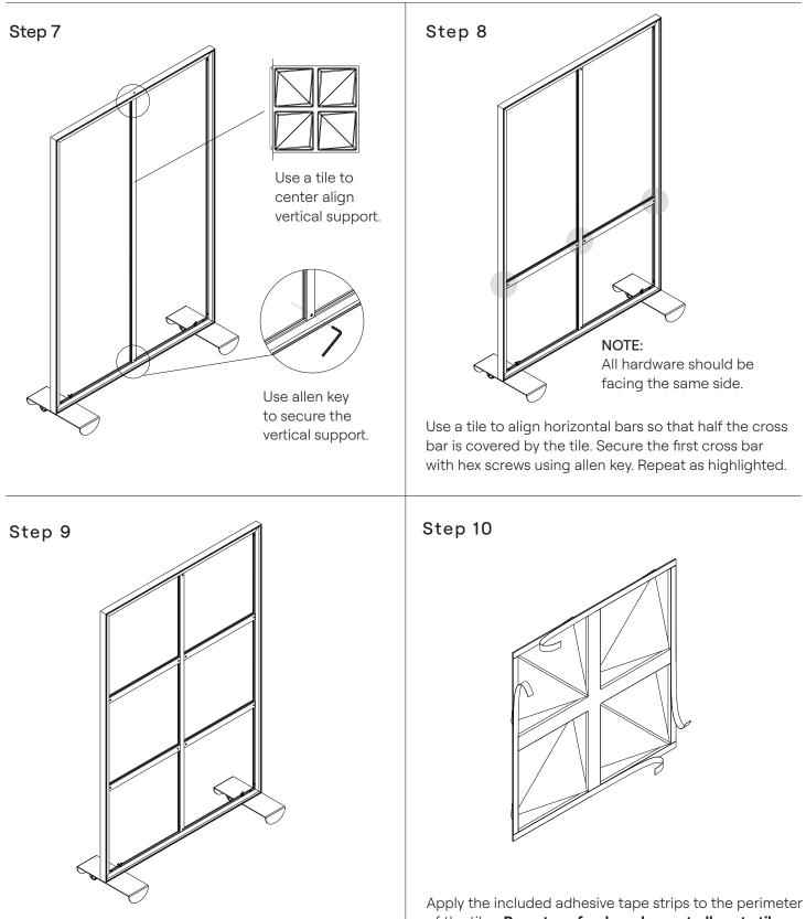
Assemble subsequent rows of horizontal supports. Ensure each tile edge has contact with the cross bars. of the tiles. **Press tape firmly and repeatedly unto tile before removing liner. Use a roller for better adhesion.**
