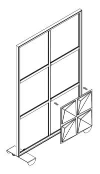
Apply tiles starting at the corner. **Press tiles firmly and** repeatedly against the frame to ensure proper adhesion to the frame. **Pro Tip:** Use the tape liner to avoid peeling. Step 12
