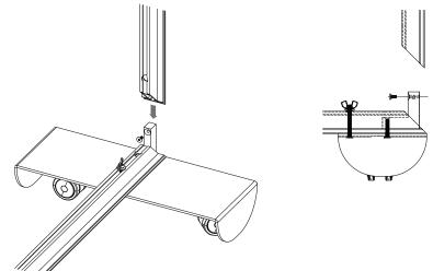
Insert the long vertical extrusion and secure with the hex screw and allen key. Repeat this step on the other side.
