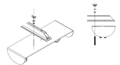
Align and secure the short extrusion with four holes at the bottom to the caster base using the long screw, wingnut and washers.
