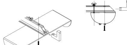
Use the shorter screw to secure the caster base into the threads in the frame.
