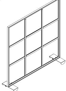
Assemble subsequent rows of horizontal supports. **Ensure each tile edge has contact with the cross bars.**
