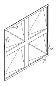
Apply the included adhesive tape strips to the perimeter of the tiles. Press tape firmly and repeatedly unto tile before removing liner. Use a roller for better adhesion.
