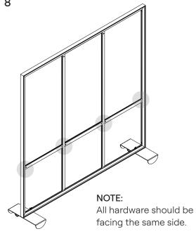
vertical support. Use a tile to align horizontal bars so that half the cross bar is covered by the tile. Secure the first cross bar with hex screws using allen key. Repeat as highlighted.
