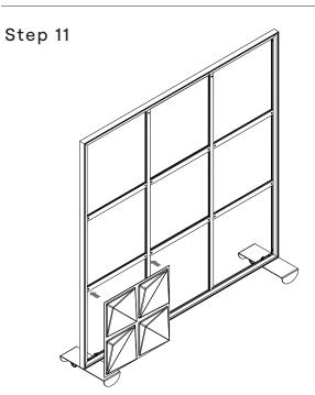
Apply tiles starting at the corner. Press tiles firmly and repeatedly against the frame to ensure proper adhesion to the frame. **Pro Tip:** Use the tape liner to avoid peeling.
