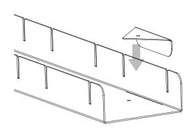
Insert caster covers as shown lining up the holes on the plate cover and the base.
