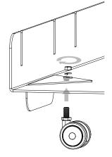
Secure plate covers by inserting the caster through the holes and securing them with the washer, lock washer and nut (in that order) 4
