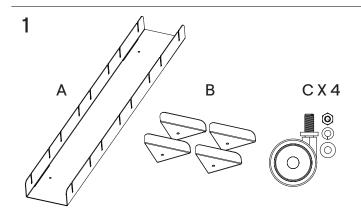
Nomad Sled includes one base (A), four wheel covers (B) and 4 casters with their respective washer, lock washer and nut.
