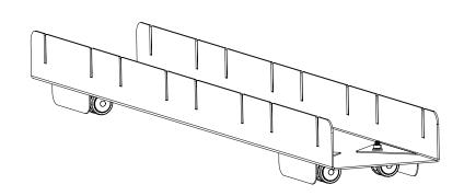
Be sure to tighten the nuts so that they are secure and check that the casters can rotate freely. The Nomad Sled is now ready to support a Nomad Felt Wall. **Use the small notches on the Nomad System Felt to secure the wall to the base.**
