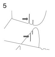
Insert subsequent rows of X assemblies into the bottom row. Use the large side slots indicated above. Repeat this step as needed.
