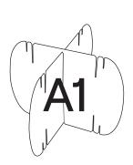
Insert one module into the other along the central slot creating the X assembly shown above. Repeat this step for each pair of modules.
