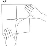
Apply tiles to surface, pressing each firmly, making sure that all corners are in contact with the surface.
