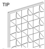
PlasticForms can be installed on a canvas or a thin plywood frame for ease of installation, transportation and finishing.
