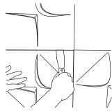
Follow the manufacturers recommended removal directions for each adhesive material. Remove tiles gently to minimize damage to surfaces.
