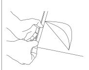
Apply the selected adhesion method to the perimeter and the center of tile when possible. We recommend 3M mounting tape.
