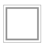
Apply a 1/4 inch adhesive bead to tile perimeter. Apply 1/4 in away from edge to prevent adhesive squeeze-out. Carefully remove and clean excess adhesive.
