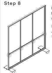
Insert one of the shorter horizontal supports and secure with hex screws using allen key.
