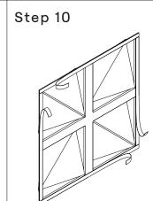
Apply the included tape to the perimeter if the tile. Press tape firmly and repeatedly unto tile before removing liner.
