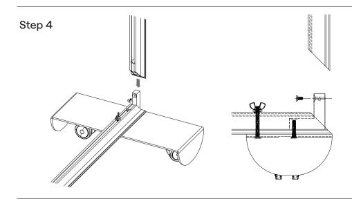
Insert the long vertical extrusion and secure with the hex screw and allen key. Repeat this step on the other side.
