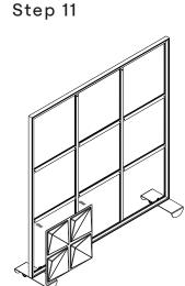
Apply tiles starting at the corner. Press tiles firmly and repeatedly against the frame to ensure proper adhesion.
