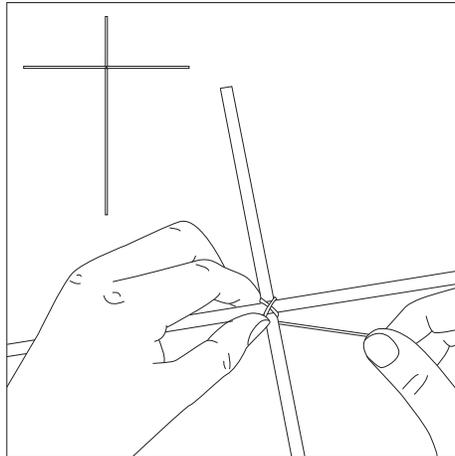
**STEP 2** Cris-cross the dowels at the markings you made earlier and wrap the string around them in an X pattern to secure them. The notches should be parallel to the ground.
