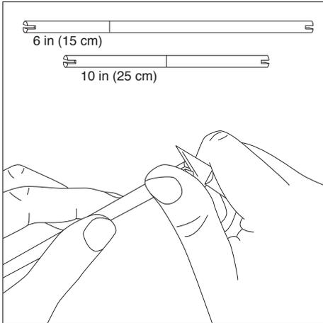
**STEP 1** Mark the 24 in (60 cm) dowel 6 in (15 cm) from the end and the 20 in (50 cm) dowel 10 in (25 cm) from the end. CAREFULLY cut notches in the ends of the dowels.
